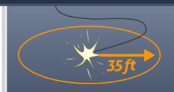
Downed power lines can energize the ground up to 35 feet away. Even more in wet conditions.
